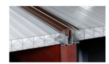
At the eaves purlin additional fixing is necessary to prevent wind uplift and downslope slippage due to repeated thermal movement. One button per sheet width, centrally located between glazing bars should be sufficient.
