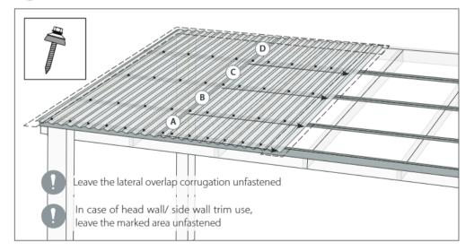
Use a butyl sealing tape between the sheet and the wall trim/ ridge cap accessory.
